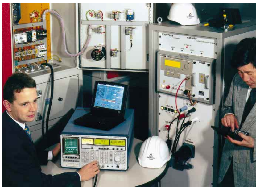
FIG 2 EMC Test Receiver ESS from Rohde & Schwarz in action at TÜV Rheinland Japan Photos: TÜV Rheinland Japan
